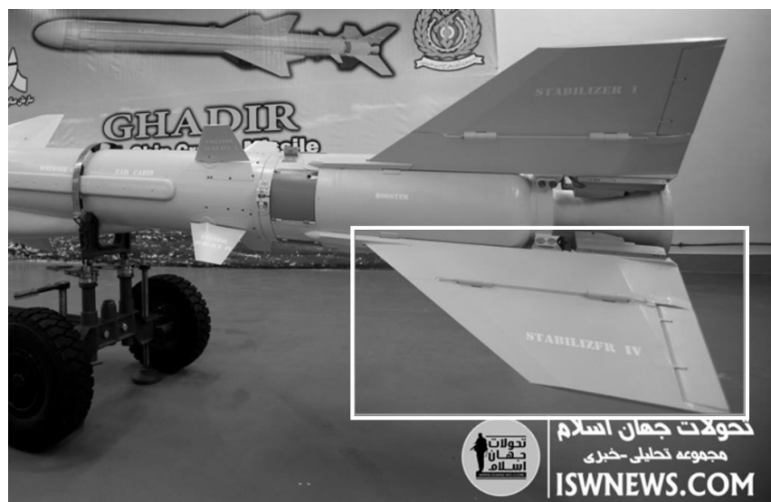
Figure 110.4 Stabilizer, Ghadir ASCM of Iranian production
