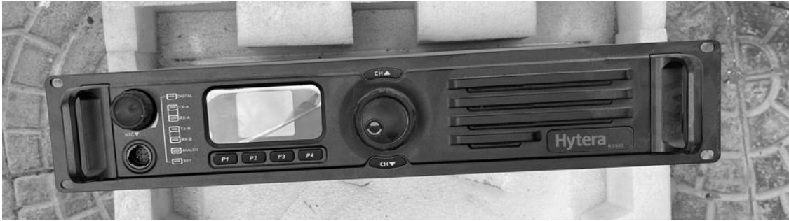
Figure 121.7 VHF station Hytera RD985
