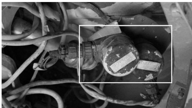
Figure 114.6 Similar pressure switches documented on an Iranian Qiam-2 debris from the attack on 8 January 2020 on a US base in Erbil, Iraq (respectively marked “GNU.D047” and “GNU.D048”) (S/2018/594, para. 90)
