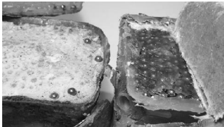
Probable C4 explosive filling with ballbearing fragmentation
