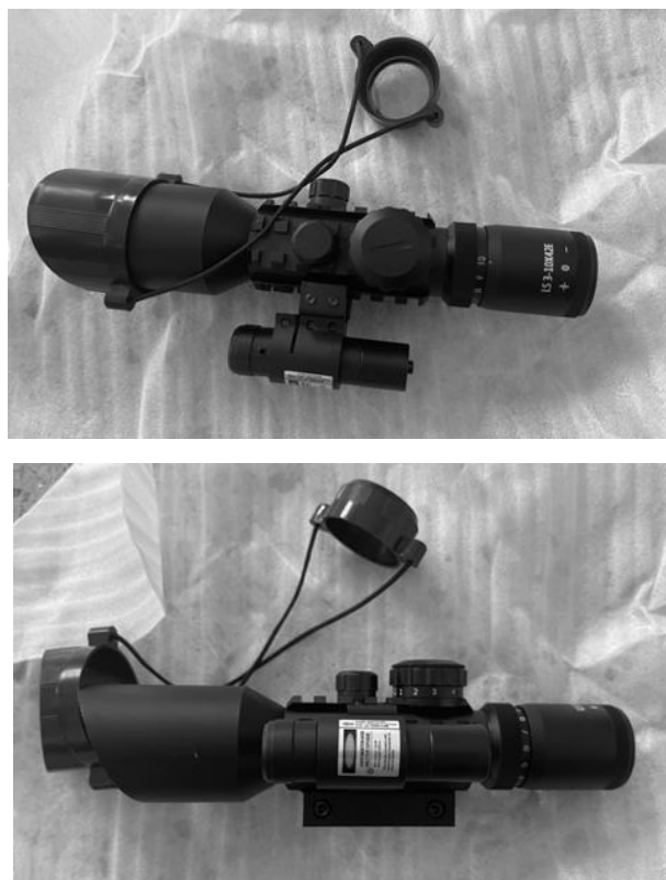
Figures 119.3 (up), and 119.4 (down) M9 LS3 3-10x42 Rifle scopes with laser sight
