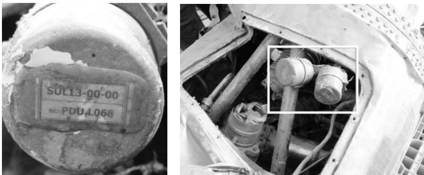
Figure 114.5 Similar markings observed on the pressure switches documented on Borkan-3 debris from attack on 7 Mar 2021 on Damman, KSA (marked “PDU.L068”)
